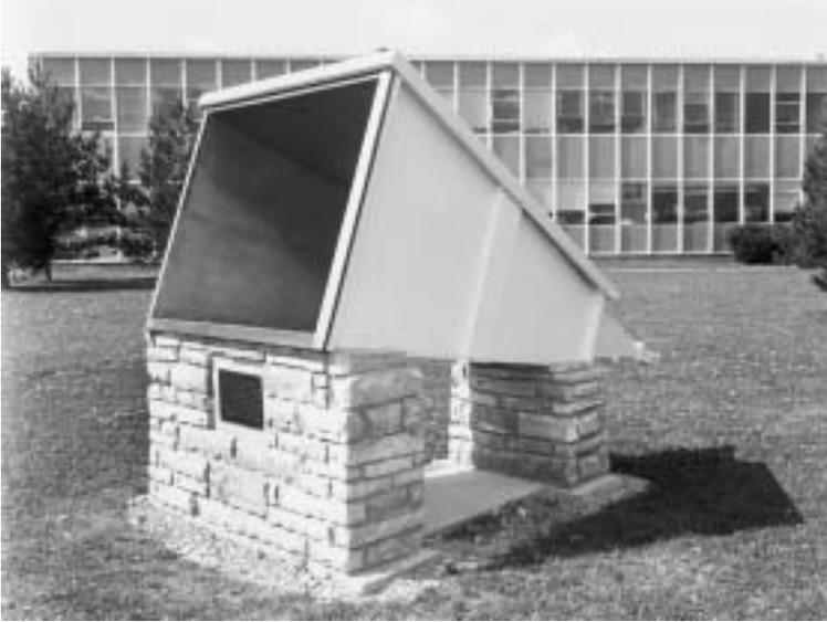
*Figure 17.2* The horn antenna used by Purcell and Ewen in their discovery of the hydrogen 21-cm line.
